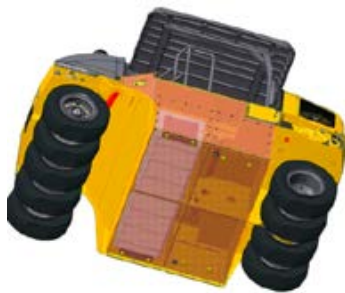
Basic unit + 7 plates 8,7 tons Basic unit + 7 plates + water 10,8 tons Basic unit + 7 plates + wet sand 12,1 tons
